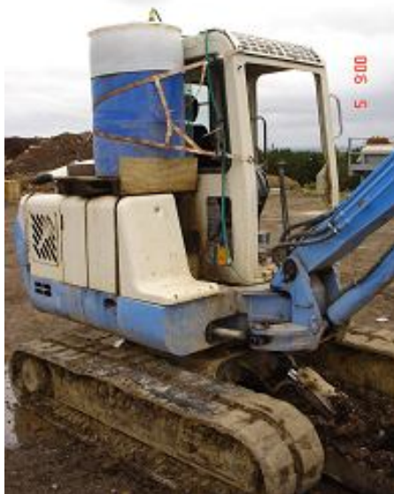
Figure 5: EM reservoir mounted on Digger Figure 6: EM dosing ring on Digger boom
