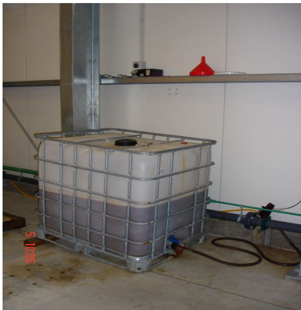
Figure 1: Reservoir containing EM plumbed to top of auger
