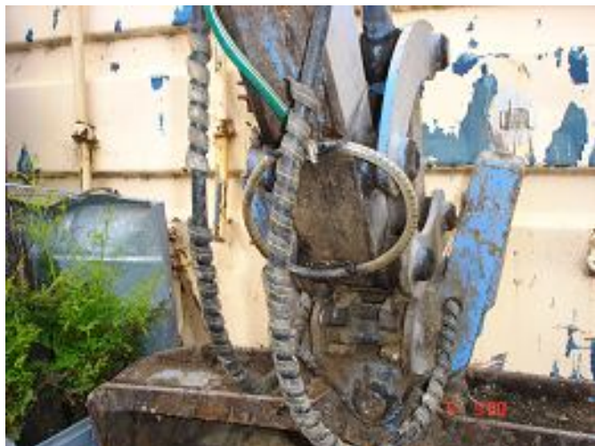
Figure 5: EM reservoir mounted on Digger Figure 6: EM dosing ring on Digger boom
