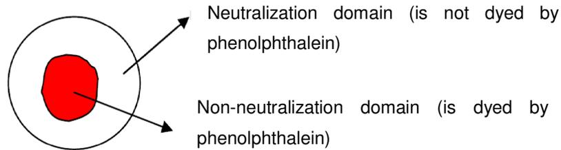
Carbonation of cylindrical test pieces
